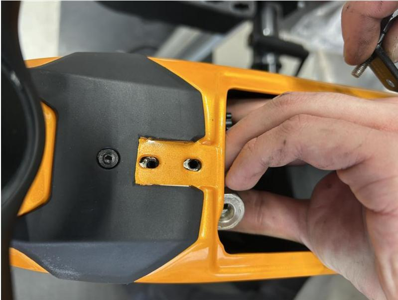
5. Reassemble the battery lock
